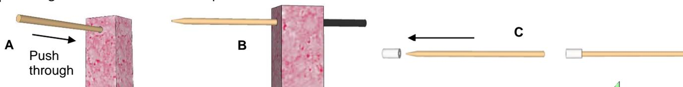
**3** Insert the tapered end of the wooden dowel into a  $\frac{3}{4}$ " long tubing section (**C**) so the tapered end reaches the end of the tubing but does not stick out.
