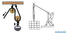
Develop super strength! A single pulley can change the direction of lifting force. Two pulleys can make lifting easier. What will happen as more pulleys are added?
