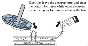
A spark can occur when the foil tab leading to the net positive charge is brought near enough to the loop leading to the net negative charge (excess electrons)
