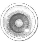
This easily-made device allows a magnet's unseen magnetic field to become "visible" in 3 dimensions. Iron filings are contained between a pair of clear lids joined at the rims and held apart by a trapped bubble of air. This simple tool can reveal the patterns due to invisible forces created by magnets.
