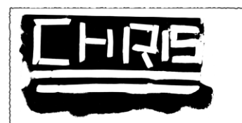
Portions of the paper exposed to heat will change color.
