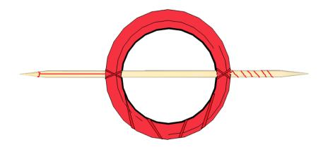
Skewer a coil of magnet wire to create a simple spinning motor! A spinning rotor needs an axle that is rigid with the ends in perfect alignment. This is difficult to arrange with wire that is flexible enough to form a coil, but automatically provided by a toothpick! The motor converts electrical energy into kinetic energy – the energy of motion.
