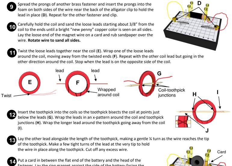
Put a card in between the flat end of the battery and the head of the fastener. Lay the ring magnet against the side of the battery facing the paperclips (see right).
