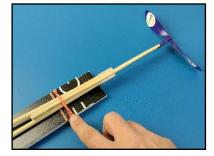
3. Rotate the beam, if needed, so the propeller's bent metal hook faces upward with respect to the chassis (see below, left). Loop the included 7" elastic band onto the hook and stretch it over the end of the beam that is protruding through the chassis, as shown below. Adjust items as needed.
