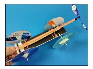
Creating a propeller power unit requires combining five different sections, listed in the table below, each satisfying a different engineering design requirement.
